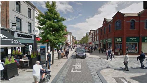
Fishergate, Preston: pedestrian priority street with narrow carriageway at level with pavement, spillout space for businesses
